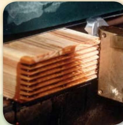
resins. OSB is made of layered wood strands oriented at right angles to develop maximum strength and stability. OSB competes with plywood and has seen significant growth due to its lower price and competitive performance in many uses. Phenol formaldehyde (PF) and, to a lesser extent, diphenyl methane diisocyanate (MDI) are
