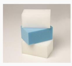
Foam manufacturers have new options when it comes to manufacturing biobased, flexible foam. Offered by Momentive Performance Materials, a surfactant called Niax\* silicone L-670 helps allow for an increased loading of natural-oil-based polyols into flexible foam.
