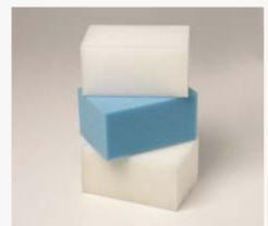
Natural oil polyols (NOPs) represent a versatile component in products ranging from foam furniture to insulation. NOPs, polyols derived from vegetable oil such as soybean oil, can replace the petrochemicals now commonly used in polyurethanes. NOPs represent one environmentally friendly option for manufacturers facing
